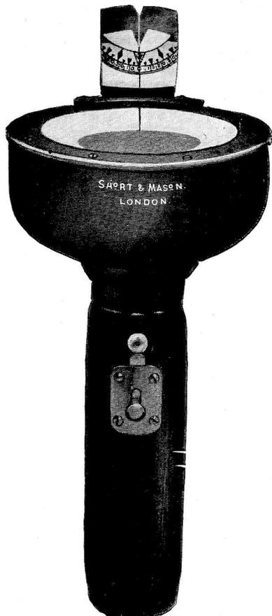
No. 1777 hand bearing prismatic liquid type, with detachable torch handle for lighting from below. Magnet system is so constructed that card will not oscillate or swing off when held or turned in taking sight. Complete in polished teak case with brass handle for carrying.
