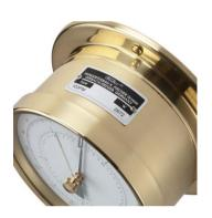
Precision aneroid barometers are used for measuring the absolute atmospheric pressure. The self-stable set of five aneroid capsules, used in our precision aneroid barometers, is made of a corrosion proof copper-beryllium-alloy. This alloy has been well established for measuring the atmospheric pressure since many years because of its remarkable elastic properties.
