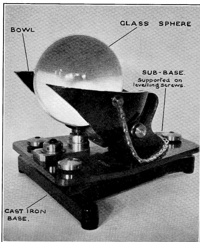
CAMPBELL-STOKES SUNSHINE RECORDER. (Meteorological Office Pattern, Mark II.)
