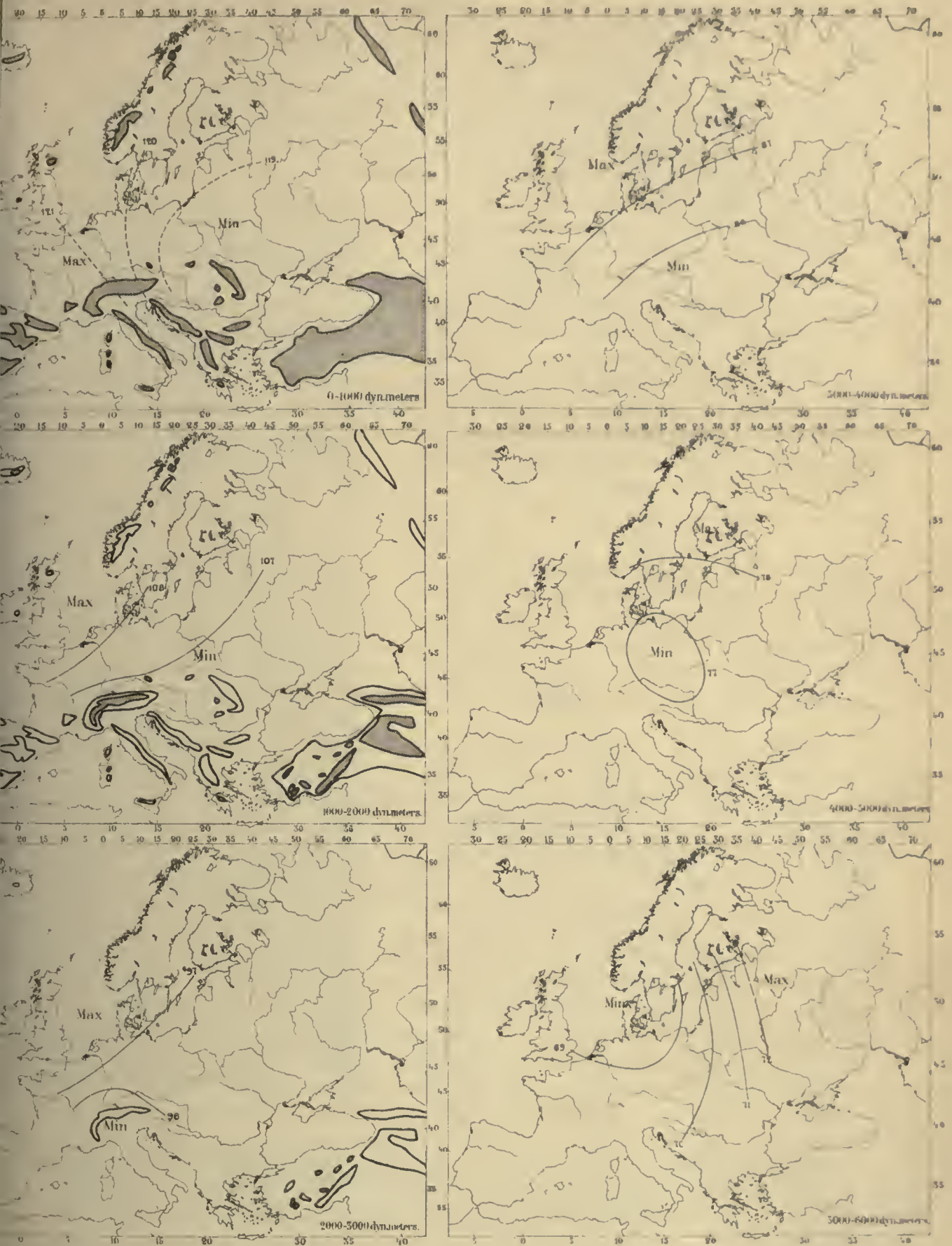
FIG. 23. Field of mass, Nov. 7, 1901, represented by charts giving the average density ( 10^{-5} ton/m 3 ) of the air between level surfaces, or the difference of pressure between these surfaces in m-bars.
