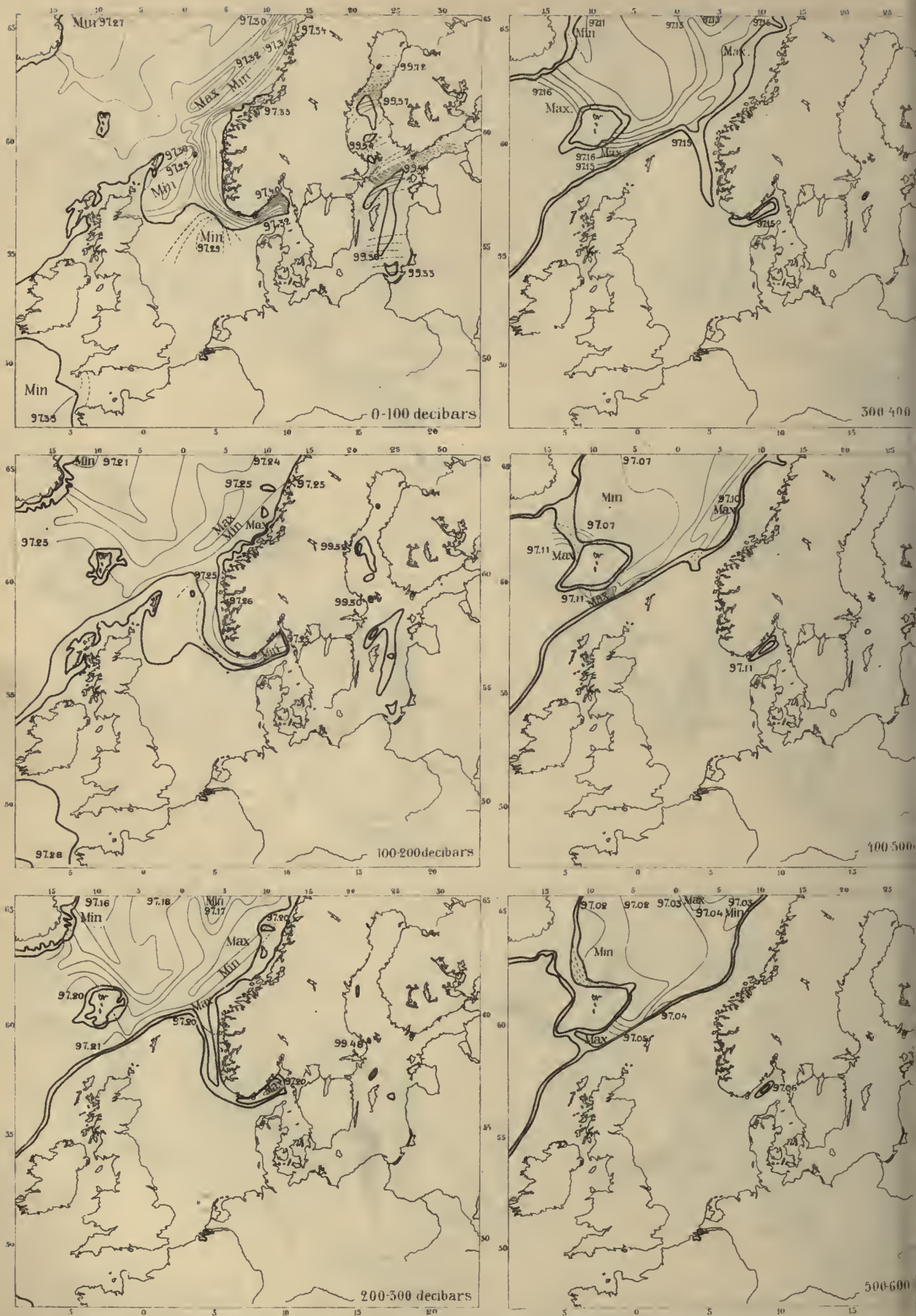
FIG. 28 (Continued). Field of mass, May, 1904, represented by charts giving the average specific volume ( 10^{-2} \text{ m}^3/\text{ton} ) of sea-water in isobaric sheets, or the thickness of these sheets in dyn. meters.
