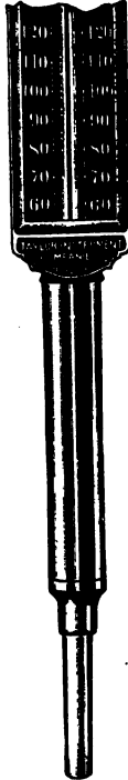
MOLTEN METAL LONG STEM. STANDARD LENGTH FORM. DIAMETER, 1\frac{1}{4} INCH. LENGTH, 18 INCHES.
