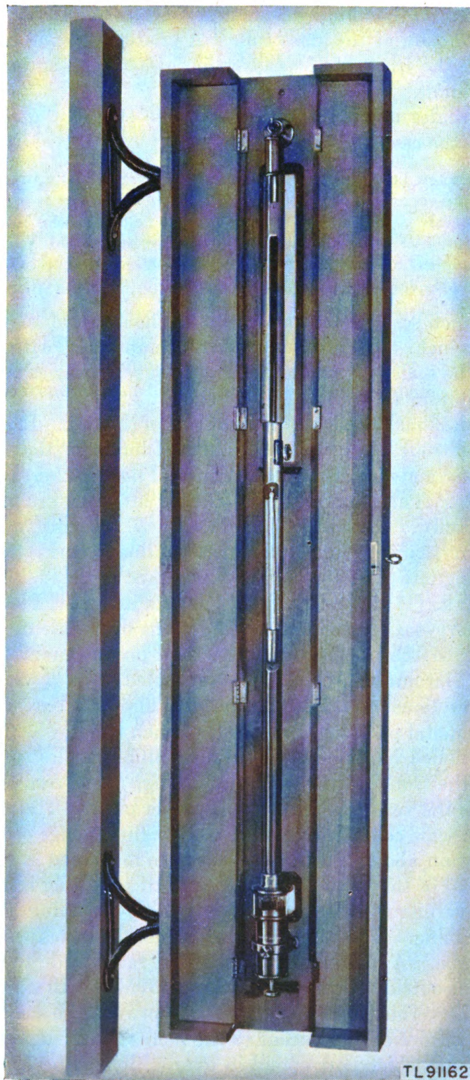
Figure 2. Barometer ML-2(*) installed in Case ML-48-(*).
