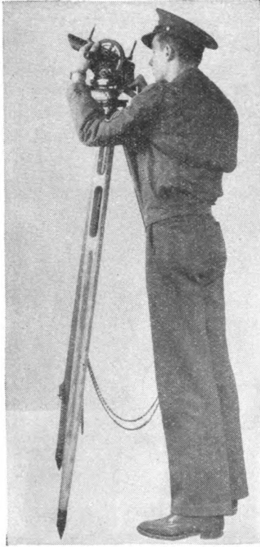
FIGURE 132.—Sighting the balloon through the gunsights.
