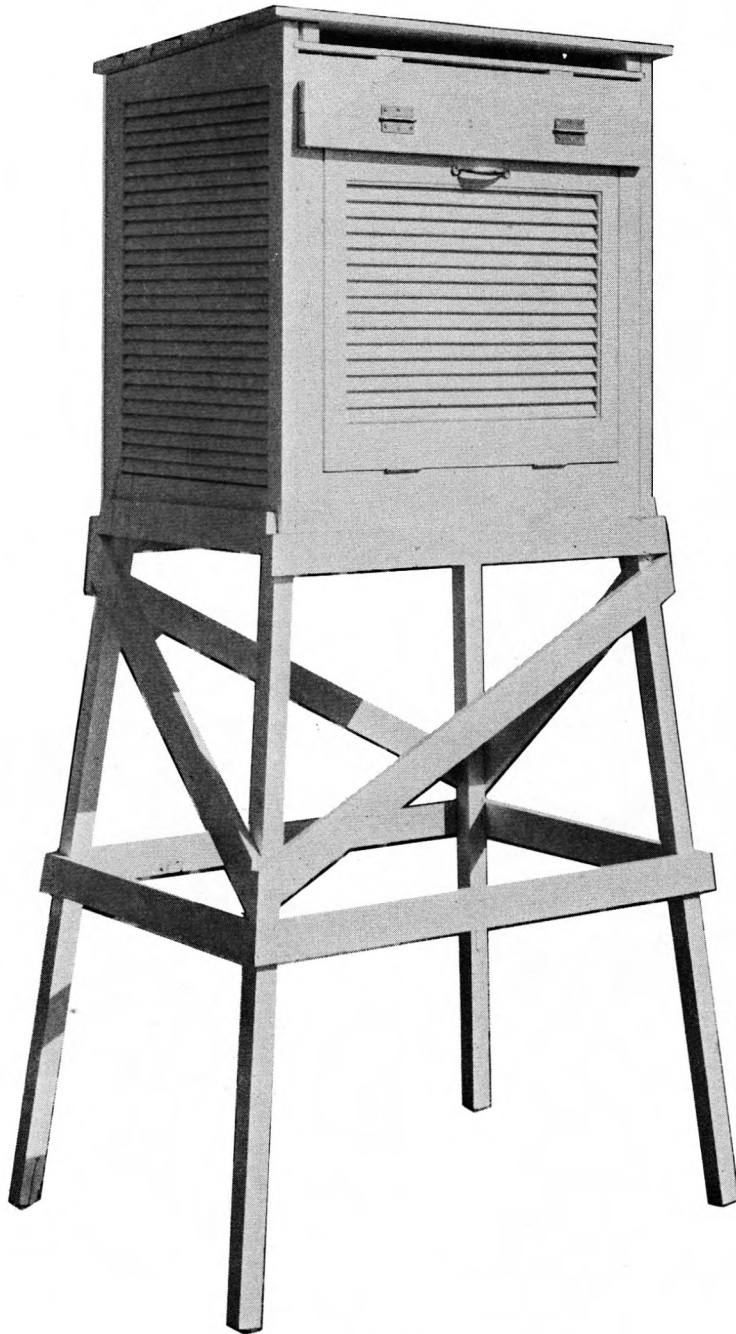
NO. 4525 INSTRUMENT SHELTER
