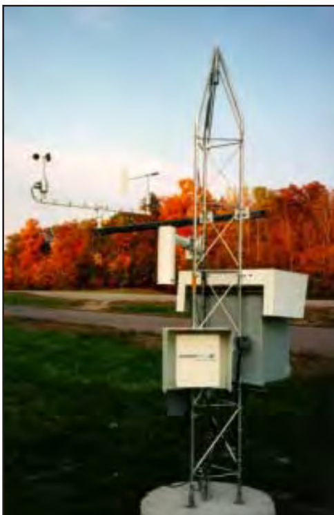
Weather Station with 10' Tower
