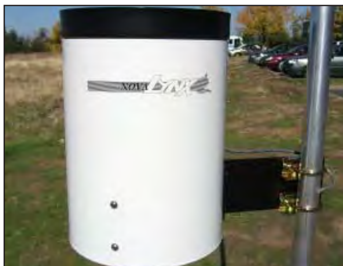
260-2501-A Rain Gauge with 260-2501MB Side Mounting Bracket
