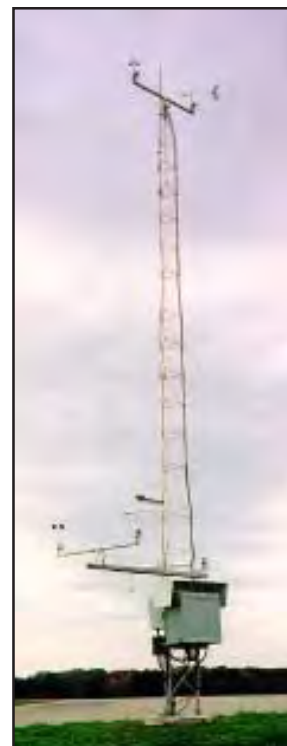
Weather Station with 30' Tower
