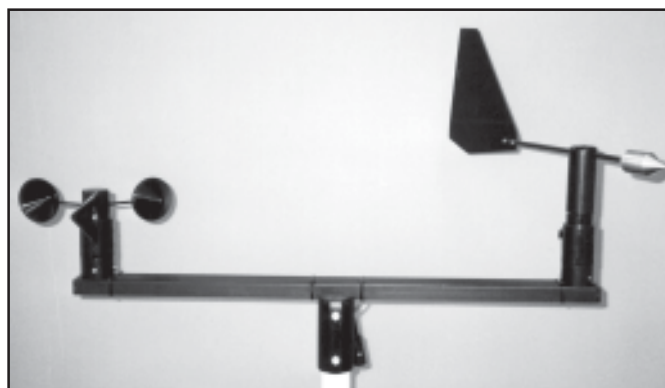
200-601 General Purpose Wind Speed & Direction Sensors on crossarm
