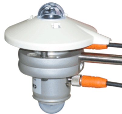
Two 240-CMP3 Pyranometers in albedometer configuration. Shown with optional 240-CMP3-MR Mounting Rod.
