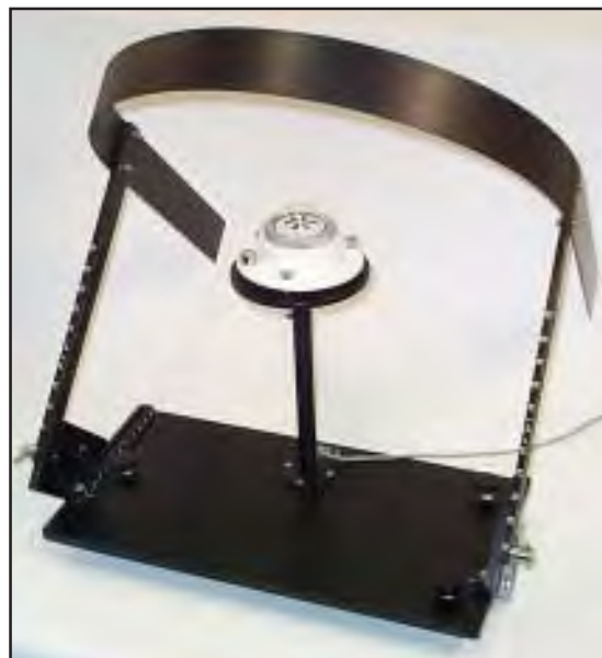
240-152 Shadow Band, shown with 240-8101 Star Pyranometer
