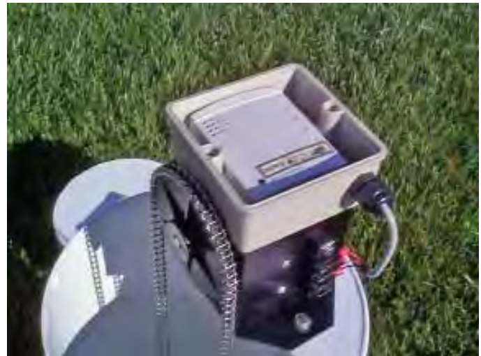
255-704-A Evaporation Logger, shown with 255-100 Evaporation Gauge
