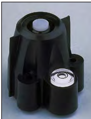
Solar Radiation Sensor
