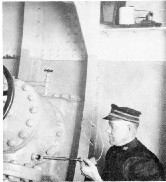
The illustration shows the Chief Engineer on the " HENRY M. FLAGLER " replacing the bulb in the pocket, and is reproduced by the courtesy of Professor Charles F. Brooks, of the Clark University, Washington, U.S.A.
