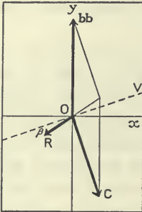
Fig. 26. The equilibrium of the frictional force of turbulence R with the pressure-gradient bb at O and the centrifugal force of the earth's rotation for the velocity V .
