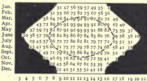
Figs. 53-56. Diurnal and seasonal variation of the intensity of solar radiation in kw/(10 m)². The broken lines indicate the points on the diagram when the altitude of the sun is 30° and when 60°.
