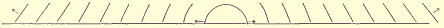
Fig. 19. Refraction of sound. Wave-fronts of a sound-wave, originally spherical, in an atmosphere in which the temperature falls off with height, but is uniform in the horizontal. The diagram is drawn approximately to scale for a change of temperature from 3000 at the surface to 2300 at 10 km.
