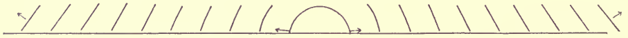
Fig. 19. Refraction of sound. Wave-fronts of a sound-wave, originally spherical, in an atmosphere in which the temperature falls off with height, but is uniform in the horizontal. The diagram is drawn approximately to scale for a change of temperature from 3000 at the surface to 2300 at 10 km.
