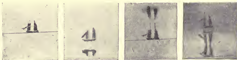
Fig. 30. Photographs of the shape of a ship through a cell of water and syrup from the positions E_4 , E_3 and E_1 . (Cp. fig. 31 a .)
