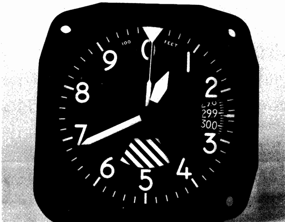
FIGURE 8.0.2. Altimeter, pressure (modified dial presentation) type MA-1. A large pointer indicates hundreds of feet and makes one revolution for each 1000 feet of altitude, and an intermediate pointer indicates thousands of feet and makes one revolution for each 10,000 feet. In addition, a small pointer indicating tens of thousands of feet is painted on a black disk with an extension line terminating in a triangular section. This provides a conspicuous indication which the pilot can use to get his approximate altitude at a quick glance. In addition, a sixty degree section marked with alternate diagonal fluorescent and black markings is provided at the bottom of the dial above the digit "5." The striped warning area is visible between zero altitude and 17,000 feet. This provides a conspicuous warning of the approach to lower altitude.
