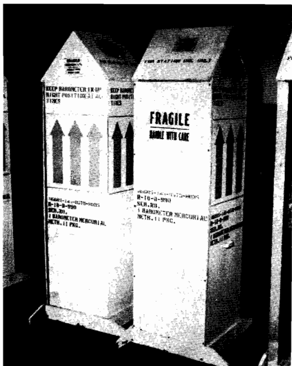
FIGURE A-2.20.6. Outer shipping boxes used by U.S. Navy for shipment of marine mercury barometers (U.S. Navy photograph). (See also figs. A-2.20.4, A-2.20.5.)
