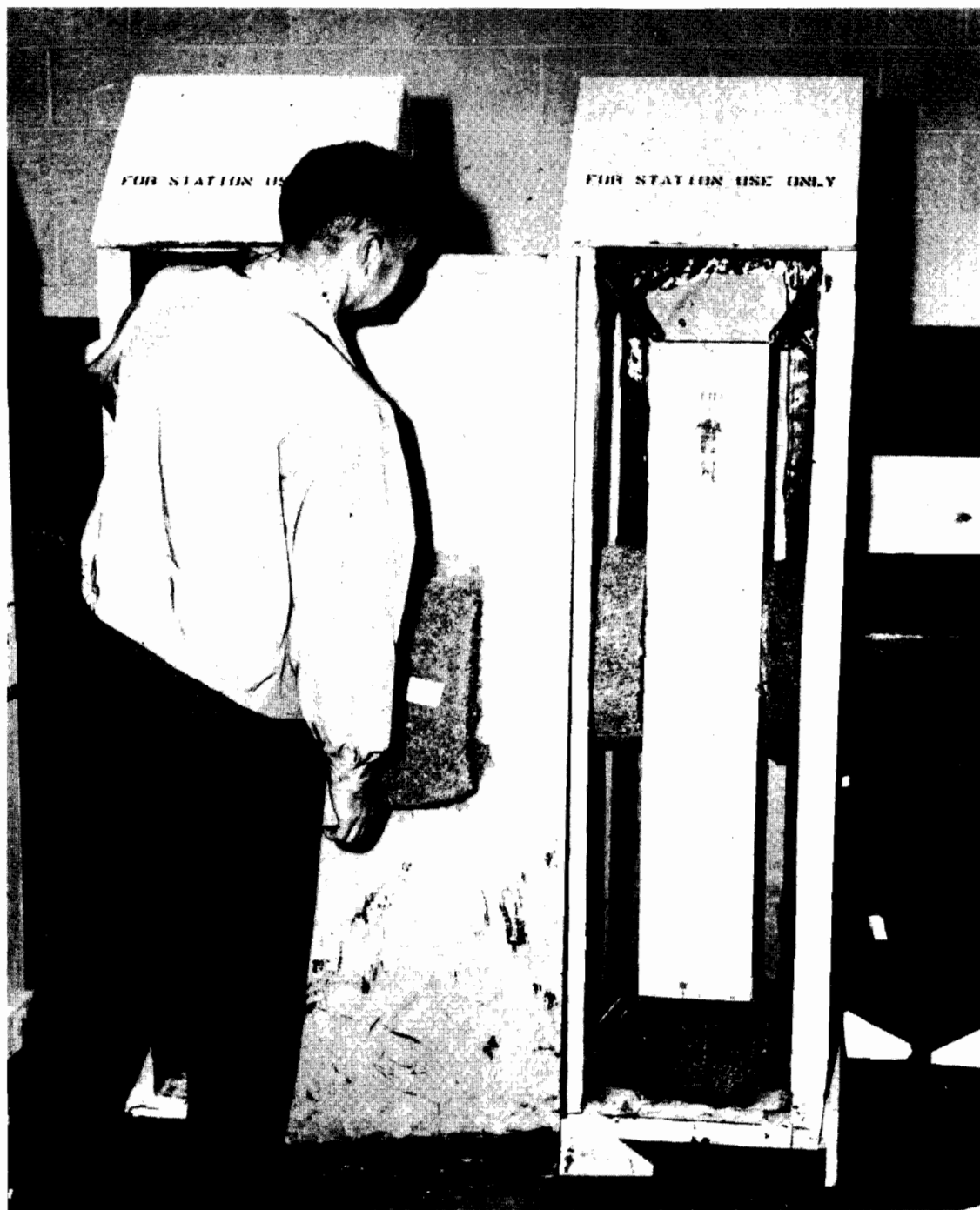
FIGURE A-2.20.4. Shipping boxes used by U.S. Navy for transportation of marine-type mercury barometers (see figs. 2.6.1, 2.6.2). Barometer is enclosed, cistern end up, in inner box which is suspended by springs and protected by wads of elastic rubberized packing material (U.S. Navy photograph).
