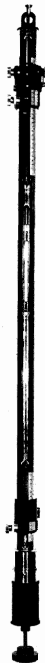
FIGURE A-2.6.1. Cistern-siphon "station barometer" designed by the firm of R. Fuess, Berlin-Steglitz. (Modified collinear U-tube type. Effective operating cross-section areas of tube and cistern are equal and the cistern is adjustable. A vernier is provided for reading position of top of upper meniscus and devices are employed for measuring heights of both lower and upper menisci. The lower sighting edge of clamping ring is fixed at zero of scale for setting lower meniscus. Range: 865—1090 mb. Bore: either 10 or 14 mm.)
