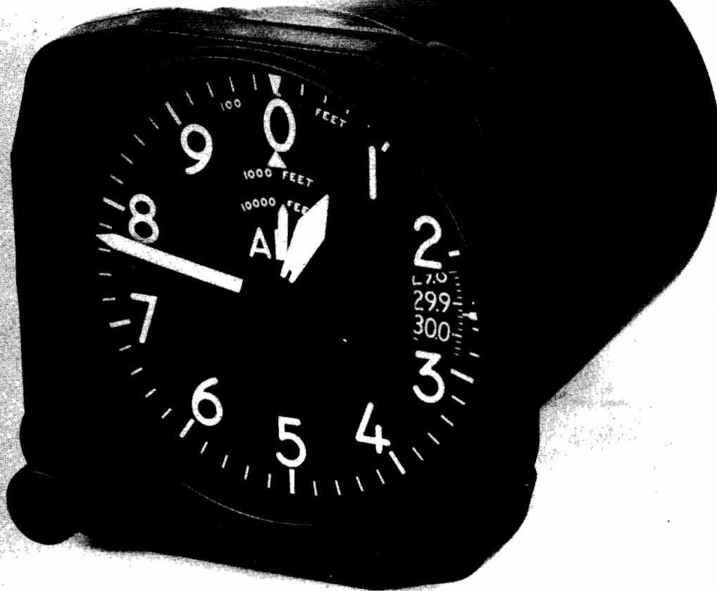
FIGURE 8.0.1. Altimeter, sensitive pressure. This illustrates the old standard altimeter having 3 concentrically mounted pointers all reading in feet with reference to a single uniformly graduated scale. A large pointer indicates hundreds of feet and makes one revolution for each 1000 feet of altitude, an intermediate pointer indicates thousands of feet and makes one revolution for each 10,000 feet, and a small pointer indicates tens of thousands of feet. The indicated altitude shown in this figure is about 800 feet. The altimeter setting scale which is controlled by a setting knob is visible through a window in the dial. The altimeter setting illustrated is 29.92 inches of mercury.
