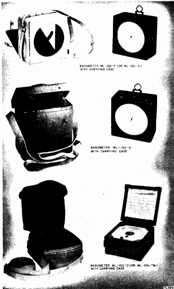
FIGURE A-2.21.5. Portable aneroid barometers ML-102-F (or ML-102-B); ML-102-E; and ML-102-D (or ML-316/TM), with carrying cases of type used by the U.S. Army and U.S. Air Force for fixed or mobile stations and for transport by hand or in vehicles (U.S. Army photograph).
