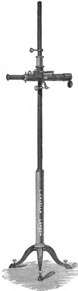
FIG. 36.—Cathetometer, 6½ feet in height.
