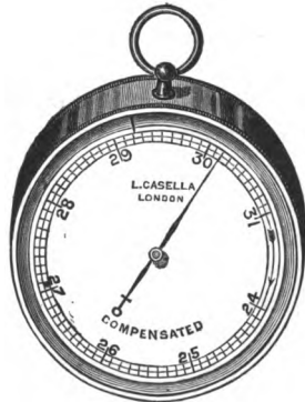
FIG. 28.—Extra-sensitive Aneroid Barometer.
