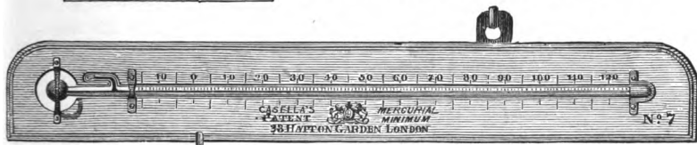
FIG. 5.—Casella's Mercurial Minimum Thermometer.
