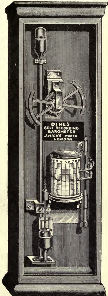
FIG. 33.—DINES'S SELF-RECORDING MERCURIAL BAROMETER.
