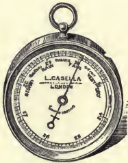
FIG. 31.—EXTRA-SENSITIVE ANEROID BAROMETER.
