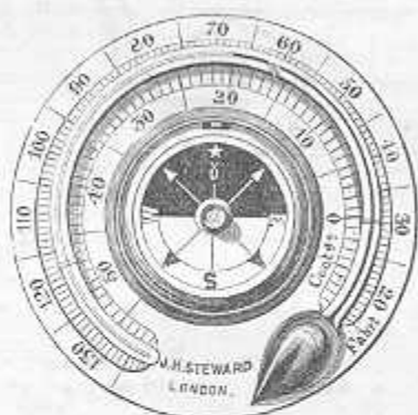
Fig. 45.—Singer's Pearl Dial Compass with Stop, and Thermometer, £1 5s.
