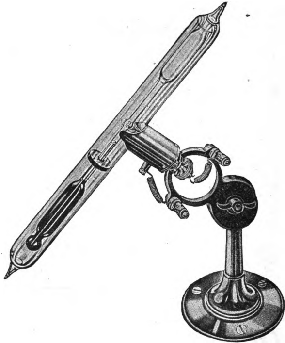
FIGURE 18. Thermometric Sunshine Recorder.
