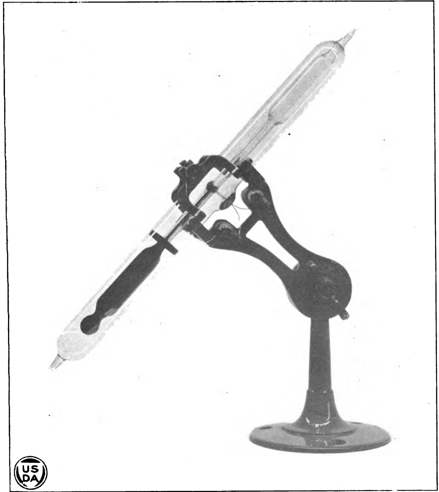
FIG. 2.—Sunshine recorder, assembled.
