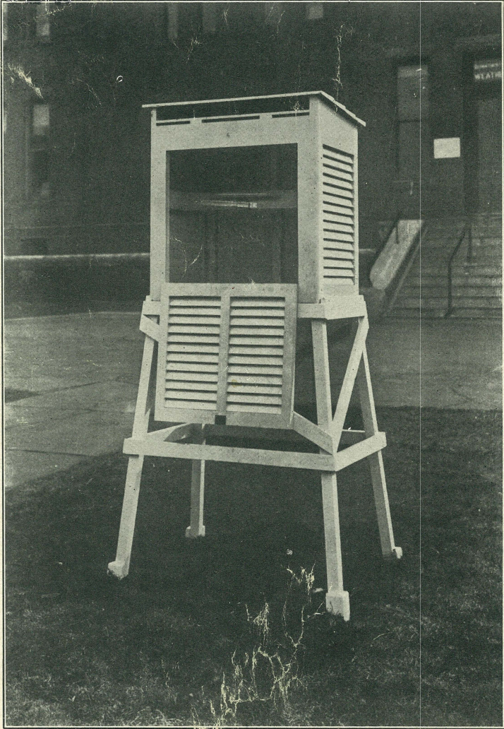
FIG. 2.—Instrument shelter on support, showing angle anchors buried in ground
