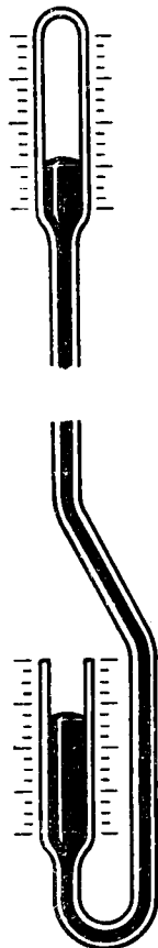
FIG. 12—PRINCIPLE OF A SIPHON BAROMETER
