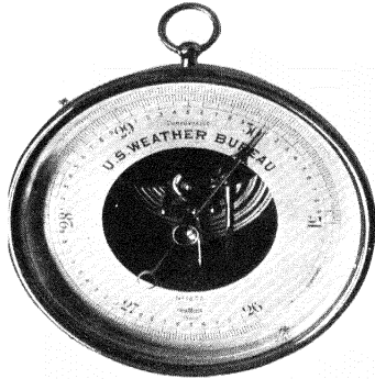
FIG. 2. ANEROID BAROMETER. This convenient portable instrument gives generally reliable indications of atmospheric pressure. Aneroids are commonly used for determinations of altitude.
