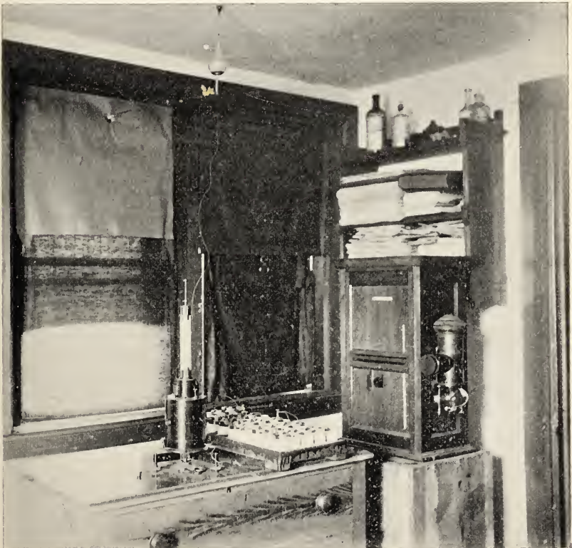
MASCART ELECTROMETER, WITH PHOTOGRAPHIC REGISTER, JULY, 1892. Blue Hill Meteorological Observatory.
