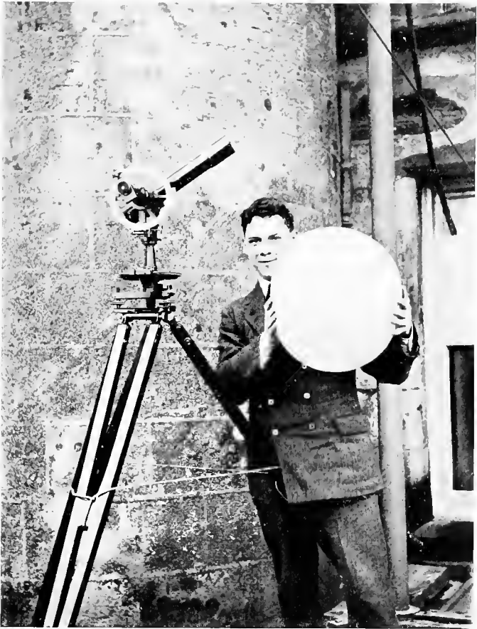
Fig. 84.—Theodolite and Pilot Balloon
